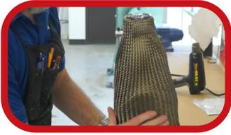
We typically use two layers of basalt, with basic nylon stockinette in different order depending on the finish, and carbon tape over the distal end.
