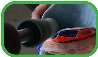
Use medium scotch bright wheel, buff outside to inside, inside to outside, smoothing and rounding off edges. when polishing and finishing Slow speed may give better results.
