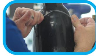
Acrylic modified epoxy resin run full vacuum at 20 to 24 in/HG until everything is saturated. When done stringing and walking away turn vacuum down to 10 to 15 in/HG.
